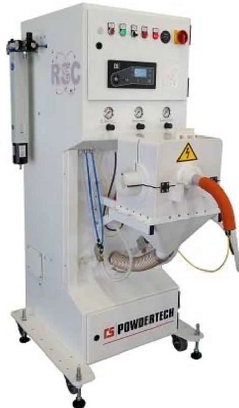
The **E-statics** is a **completely new development** and corresponds to the state of the art in surface coating technology. It shows a reduction in wear parts in the pistol as well as a longer service life of the cascade and continuously high voltage and therefore reliable charging without losses. The cascade is designed so that the full nominal output is available even on two to four pistols.
